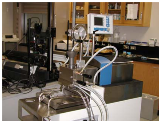
Haake PolyDrive batch mixer with on-line torque measurement
